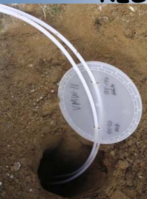
Photograph of one vapor monitoring well with two soil vapor probes.
